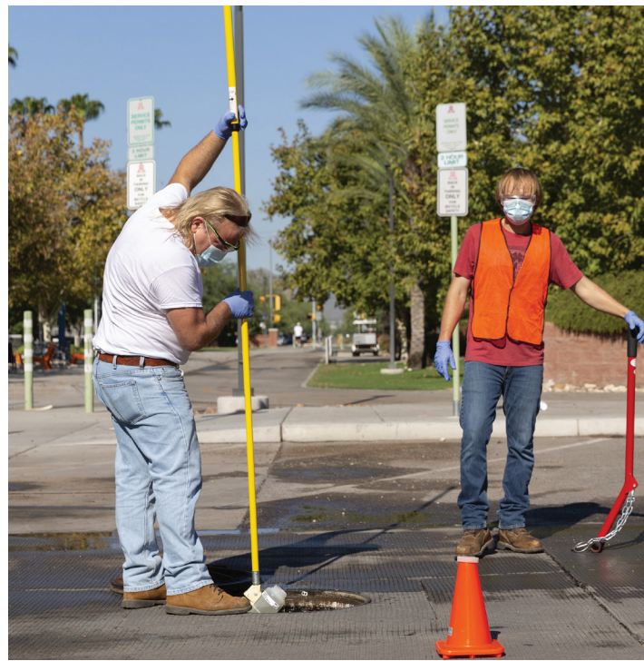
Collecting a wastewater sample from a dorm’s sewer line at the University of Arizona, August 2020.
