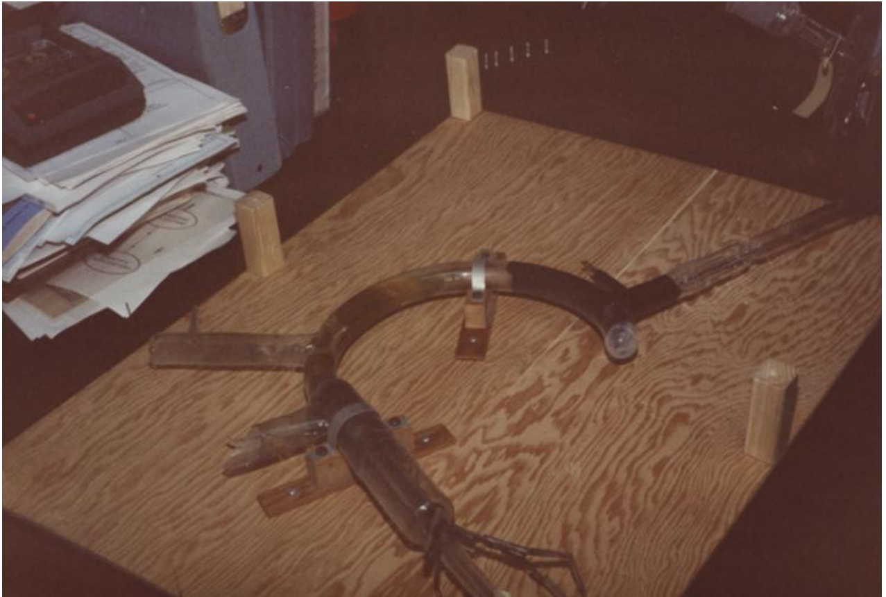
Figure 41. 180° mass spectrometer constructed at Harvard, 1937-1938.
