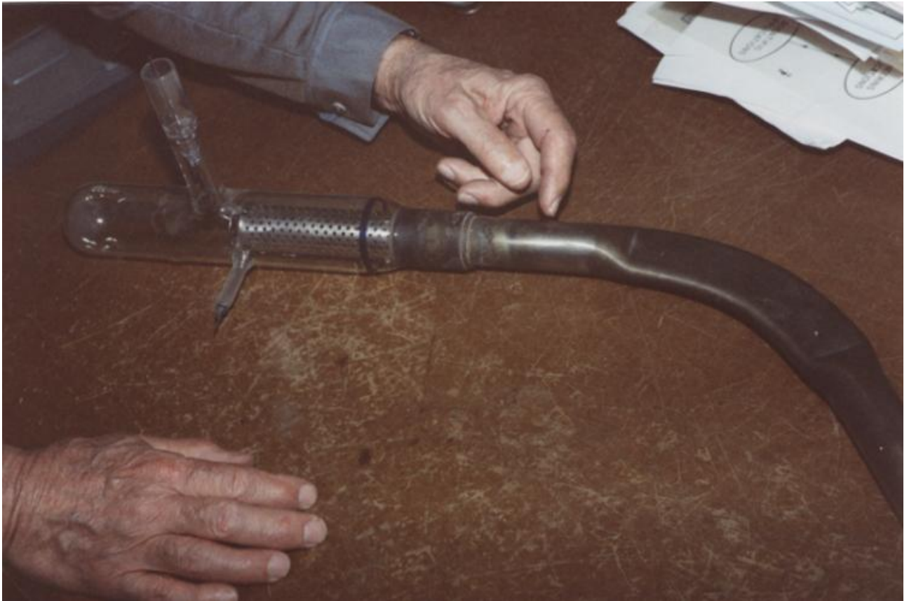
Figure 45. Collector end of early 60° tube. Note Kovar seal joint where glass housing over collector plates joins copper flight tube.
