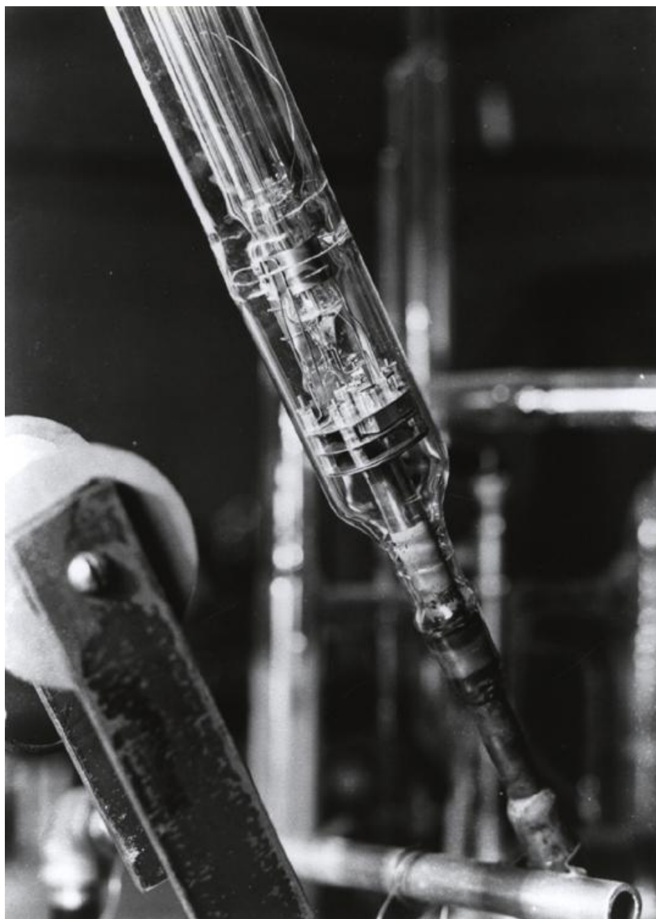
Figure 11. Ion source for early 60° mass spectrometer (circa 1941).
