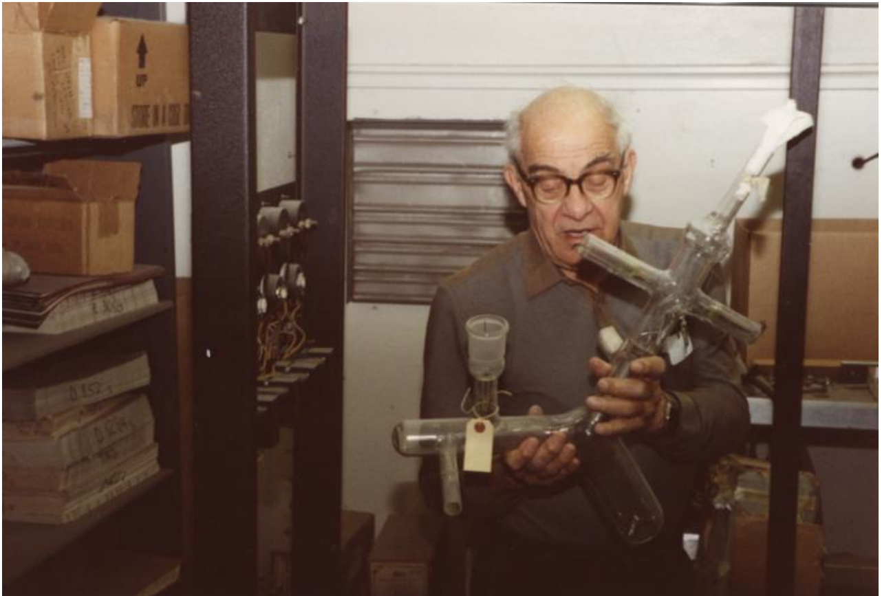
Figure 15. Spare hydrogen isotope mass spectrometer tube with internal permanent magnets. Constructed 1942-1943.
