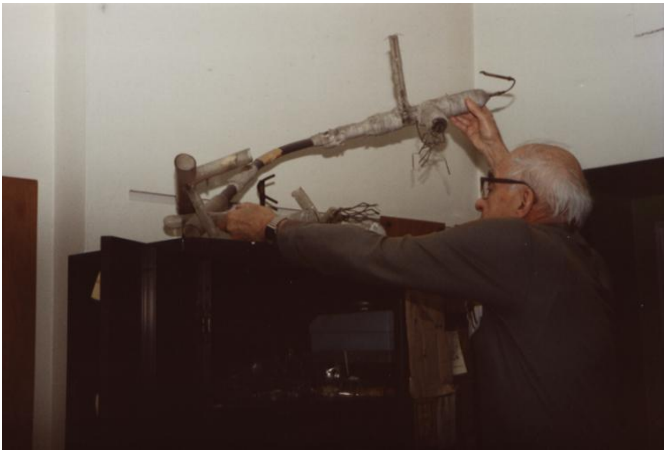
Figure 39. One of several early 60^\circ mass spectrometer tubes constructed in 1941-1942 period.
