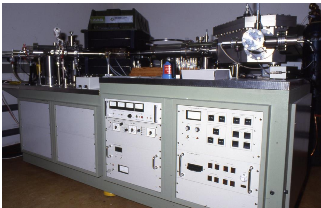
Figure 6. Tube unit from the VG Micromass ZAB 2HF double focusing instrument
